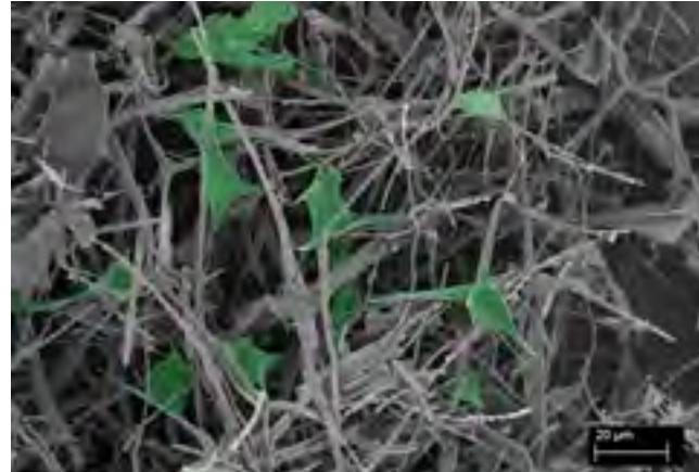
Figure 3: Scanning electron microscopy image of fibroblast cells (green) adhering to aerographite microfibers (Lamprecht et al., 2016).
